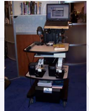
Shelf Reading Wand and System on Cart (Model shown includes Total Mobile Complete Staff station with Tag programming and dispensing and Inventory)
